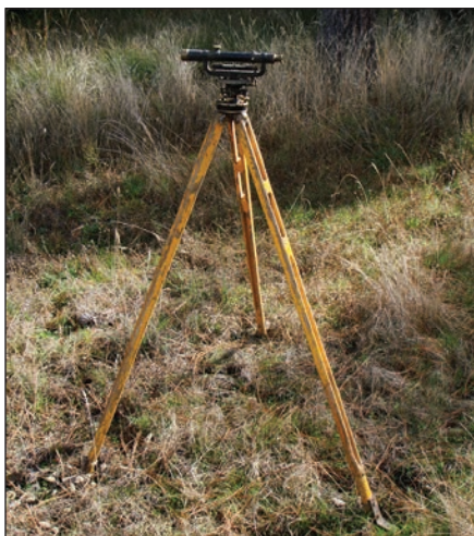
A tripod and level are needed to determine slope when installing culverts or road grades.
