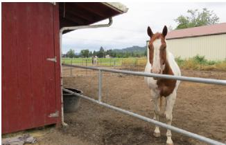
Photo: Melissa Fery, © Oregon State University Figure 16. Gutters and downspouts reduce mud by directing water away from high-use areas.
